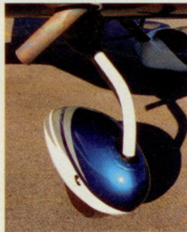
The backseats are cozy but comfortable (above). Differential braking is used to steer the full-castering nosewheel (right).
